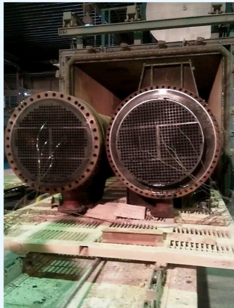
Step 5 Safely clean all parts with our advanced thermal cleaning process
