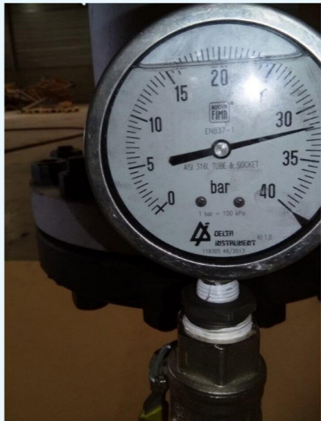
Step 8 Pressure testing to verify the heat exchanger is 100% operational and to detect any potential leakage
