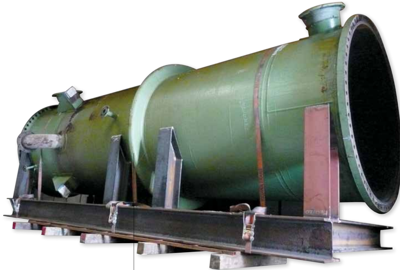
HEAT EXCHANGER WITH COMPENSATOR
